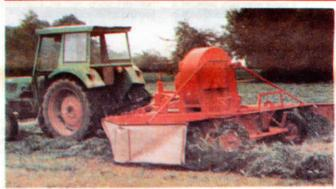
New machine "blows" cut hay into two windrows. Air blasts out of narrow opening just above ground surface (see photo below).
