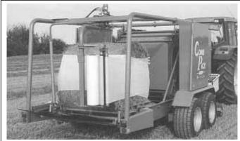
Krone's new "Combi Pack" bale and wrap machine is built as a single piece of equipment for baling and wrapping in one operation. It's based on the company's Round Pack baler which has a built-in chopping unit.
