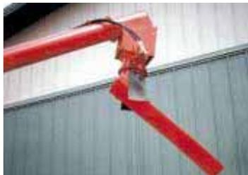
Hydraulic-operated grain spout can be rotated 360 degrees to any position.
