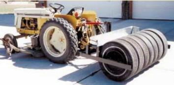
Mueller pulls rubber-tired roller behind tractor when mowing. Weed seeds with burs stick to wheels and are collected in hopper for disposal.
