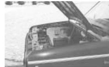
**Pickup now has 20 6-volt batteries under the hood and 14 back in the bed.**
