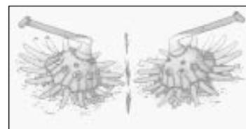
**The In-Row Weeder is a 7-in. cone-shaped wheel with 3 1/2-in. long rubber fingers for weeding.**
