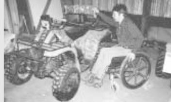
a Polaris ATV. It has all hand controls and a special high back support, which he "padded" with camouflaged tape. He can get on and off the ATV by himself.
