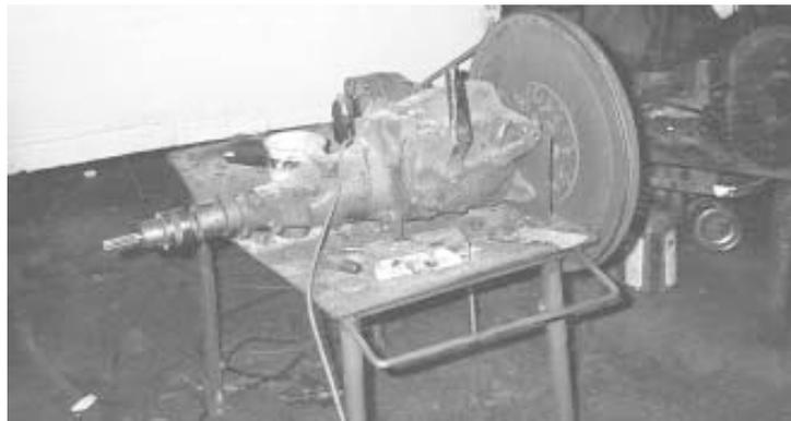
**Knafelc fitted an adjustable chuck to transmission's output shaft, to hold taps and dies for cutting threads. Transmission is belt-driven by a 1/4 hp electric motor.**
