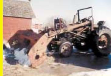
moved the reel, auger, feederhouse chains, and guards. The bucket is tilted by the loader's original cylinders. It really works great for scooping snow out of our yard and can pick up three cubic yards at a time. That's about three times as much as a standard Du-All bucket can hold. It's also built tough - one time I caught the bucket so hard on something that it stopped the tractor, but the bucket wasn't damaged at all. **(Stan Knafelc, Box 67, Watson, Sask., Canada S0K 4V0 ph 306 287-3789)**
