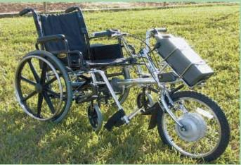
Add-on front fork is powered by an electric motor and battery pack. It attaches to virtually any standard folding or sports wheelchair.
