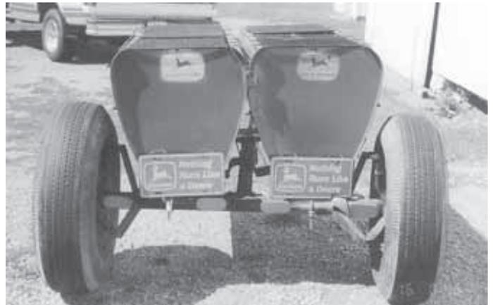
Barbeque was made out of a pair of fertilizer boxes off an old corn planter, with wheels and a hitch added so Hoehn can take the double grill anywhere.
