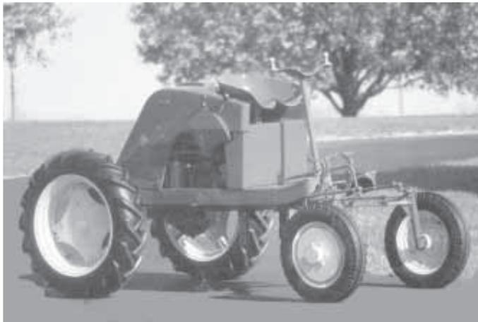
Deere's experimental "No. 101", owned by Ron and Barb Koogler, was one of only five units built. It was designed to provide an unobstructed view both ahead and behind.
