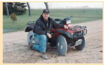
Steel "trench wheels" for ATV's are a great new way to drain excess water from fields without damaging much of the crop, says inventor Steve Raguse.
