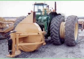
Schnack stripped a Kools silage blower down to the star wheel, pto shaft and bearings.
