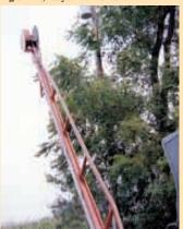
Mounting the saw on the skid steer arms allows Brenneman to raise saw nearly 25 ft. high.
