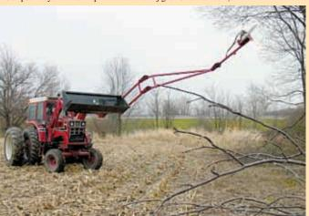
The "A.R.M." is a 15-ft., foldable arm that adapts a Stihl chain saw to a front-end loader. It can reach up to 30-ft. high branches when it's fully extended.
