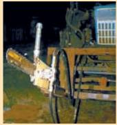
Hydraulic-powered chain saw slips on and off the forks on Ronnie Campbell's frontend loader.
