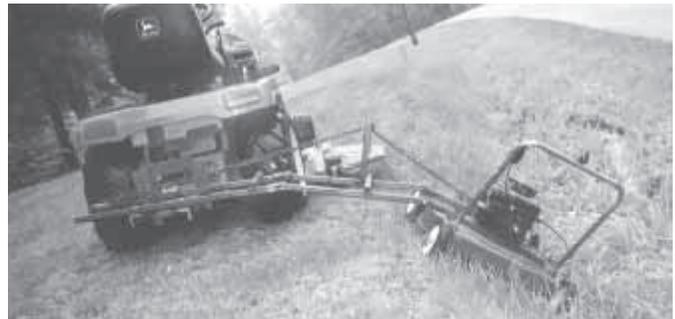
Homemade flexible hitch allows Chris Rahman to pull a 22-in. push mower 2 ft. to the side of his Deere garden tractor.
