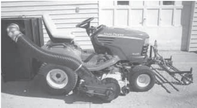
"I use it to pick up and grind leaves around my house," says Pat Prom about the blower-vacuum he made to fit his garden tractor fitted with a mower.
