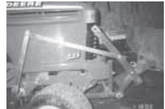
Rahman mounted a 42-in. Snapper blade on front of tractor. A rod bolted to the hydraulic deck lift mechanism on tractor is used to raise and lower blade.
