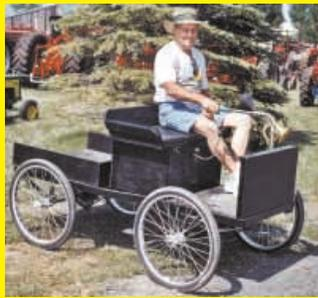
of plywood over a frame made from 1 by 2-in. rectangular tubing. The vehicle has tiller steering and a squeeze bulb horn on front, and a small wooden box on back. The vehicle's 8 hp Briggs & Stratton engine and 5-speed transmission are out of a 1968 Deere riding mower.
