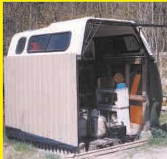
to the outside of the skids and added some caulking to make the shelter water-tight. By setting the walls on a 2 by 6 bottom plate, I can use a truck or tractor to tow the building to a new location. (Louis Trepanier, Rt. 2, Haliburton, Ontario, Canada KOM 1S0)
