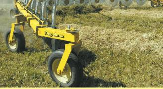
High-capacity wheel rake has oversized wheels and an overall beefier frame.
