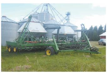
Tom McMillan wanted to apply all his fertilizer at once, as dry product, with one machine. To accomplish that, he replaced the original seed and fertilizer boxes on his Deere 752 no-till drill with two used 110-bu. tanks off a Flexi-coil air seeder.
