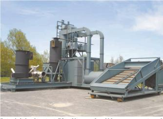
System is designed to extract oil from biomass such as chicken manure or waste wood, at the same time producing a beneficial fertilizer product. It works by vaporizing and condensing the biomass in the absence of air.
