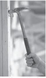
Hammer's front-mounted claw pulls 12 to 20-penny nails with no need to flip the hammer over.
