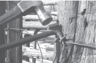
Staple puller has a long point at one end with a flat driving plate behind it. You position point between post and staple and use a hammer to drive it in.
