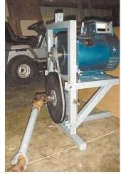
Madison found a generator on eBay and made a frame to pto-power it on a 3-pt. hitch.
