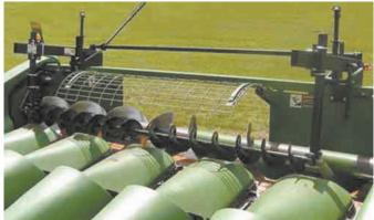
Auger attaches to Deere 90 series corn head frame using clamp-type fasteners. The system is self-contained and operates off a hydraulic motor.
