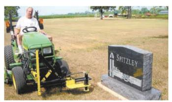
Spitzley used scrap parts to build the string trimmer. "From the seat of the tractor, the head can be adjusted 1 ft. in any direction," he says.
