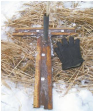
Fence post drops into a short pipe welded to a base made from welded-together grader blades. Post holders are heavy enough to allow an 80-ft. span between posts.
