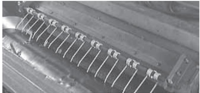
“The Buck Stops Here” attachment fits onto combine feederhouse, tearing weeds off header auger before they start to wrap.
