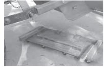
Len Pautz came up with this rolling cart that fastens to the bottom of his 60-in. snowblower. Cart is made from 1/2-in. thick plywood and rides on 8 small wheels.
