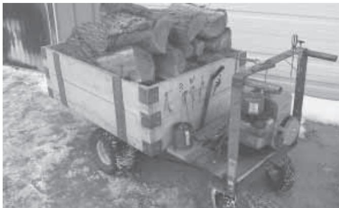
Wheelbarrow is driven by a 5 hp engine. Caster wheels on back allow short turns.
