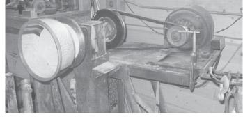
Warnecke made his own lathe. One of its main component is a flywheel off an old Datsun, which serves as a weighted pulley.
