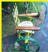
wagon, with leaf springs welded onto the bottom. The armrests are made from stained wood, and the back was made by cutting down a steel gate. There's a cup holder on one side. (George Feltz, 6280 5th St., Stevens Point, Wis. 54482, ph 715 341-0162)
