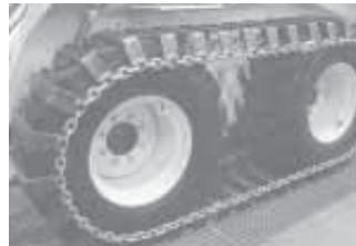
two wheels on either side of the loader. The tracks are held together by lengths of log chain which the company says gives them tremendous strength. “We like the web spacing and good combination of float and bite,” says Chad, who runs a concrete company that does concrete foundations, concrete repair, and other work. “We’re often dealing with mud and sloppy conditions. That’s where the Eel Trax pay off.”
