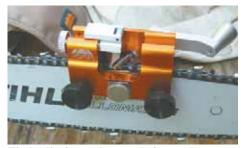
Timberline's crank-type chainsaw sharpener comes with a carbide cutter that rides the bar. The operator pulls the chain through to sharpen each tooth.
