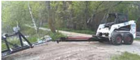
Telescoping hitch made it easy to put pontoon boat into water on a steep landing.
