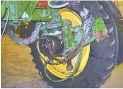
Photo above and at left shows Deere 4930 sprayer being fitted with new ATC electric drive wheel motors.
