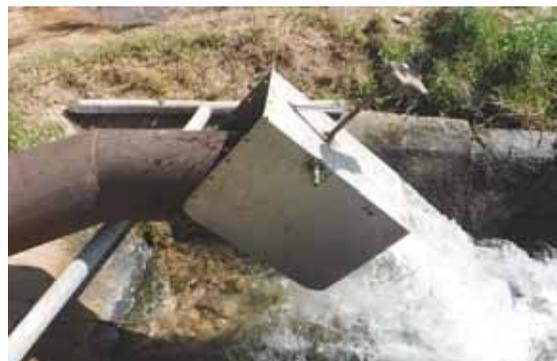
“Coon preventer” spout automatically opens with moving water and closes when water stops flowing.
