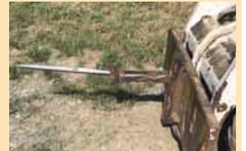
Zigler slips a pto shield over his bale spear, bell end out. It lets him pull spear out without messing up the stack.
