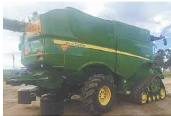
"Chaff Deck" uses enclosed conveyor belts on back of combine to drop chaff onto the wheel tracks, instead of spreading it out over a wider area.
