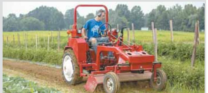
Soon to be introduced items include a modular rotary hoe (above) and a parallel cultivator.
