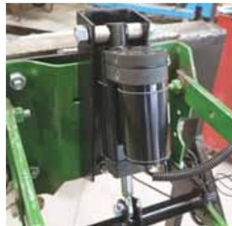
Electronic depth control kit for planters combines an electric actuator with a self-contained hydraulic chamber.
