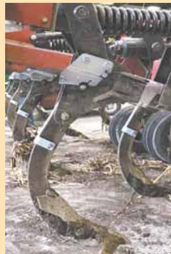
“Shear bolt monitor” lets you know right away when a shear bolt is broken so you can get that shank working again.
