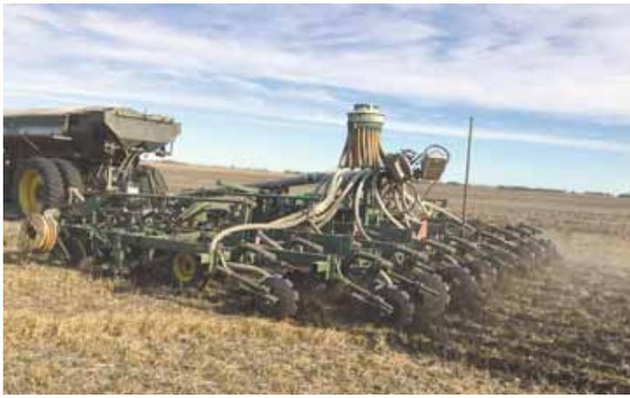
Don Bot and son Chad use a salvaged fertilizer cart to supply their home-built, 18-row strip tiller equipped with an airflow distribution tower.
