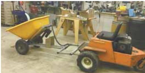
John Houston converted an old Woods zero-turn riding mower into this powered wheelbarrow. "Works well for dumping concrete," he says.
