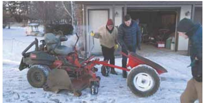
Allen Hernke uses his zero-turn riding mower to push a modified wheelbarrow. He replaced wheelbarrow's front wheel with an axle and two 15-in. wheels.
