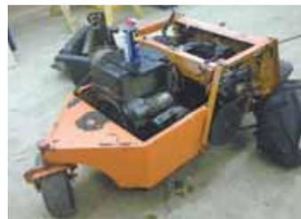
He stripped down the mower, then built a pivot point on front that allows wheelbarrow to float up or down.
