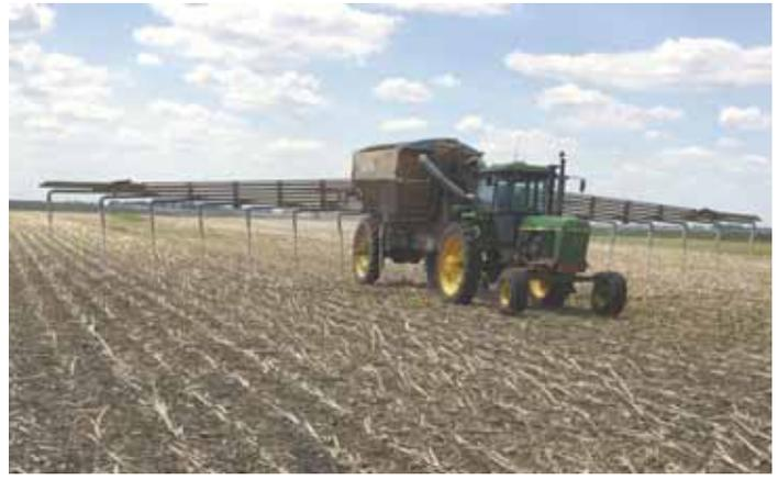
Side-dress applicator with airflow boom and distribution system is mounted on front of a salvaged fertilizer spreader box.
