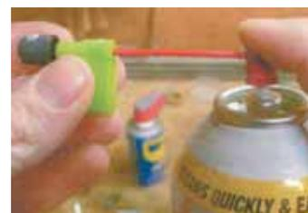
**Spray Can Tool is designed to adapt most common spray can applicator tips to the applicator straw on an aerosol can of carburetor cleaner.**
