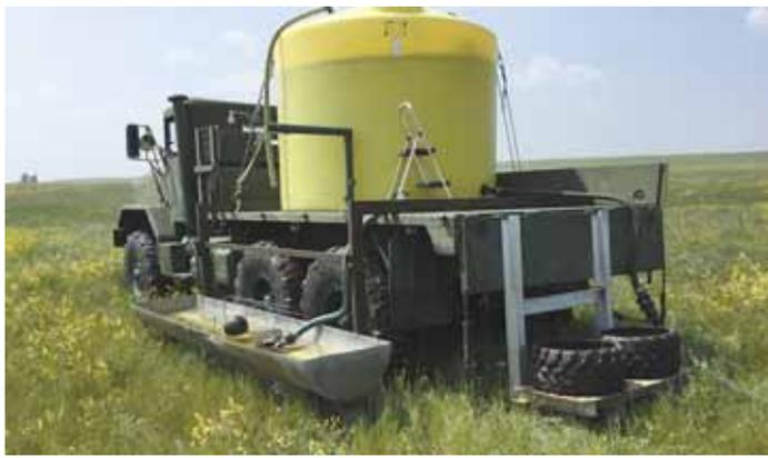
Jeff Brown made this portable water rig using an old Army 6 by 6 truck. The 2,000-gal. poly tank delivers water to a trough along the side.
