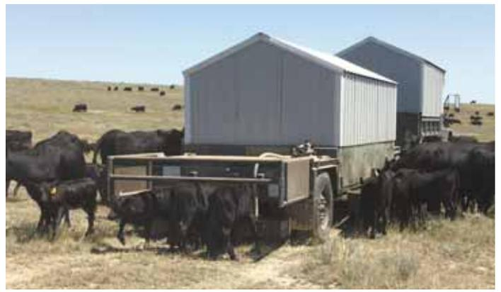
He used the same idea on an old military trailer pulled behind the truck. Photo shows small sheds he added later to cover the tanks to keep slime from forming inside tanks.
