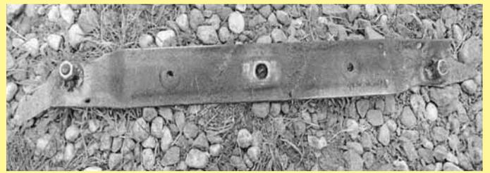
Bug Vogelzang modified his mower blades with swinging sickle sections on each end to cut through heavy grass.
