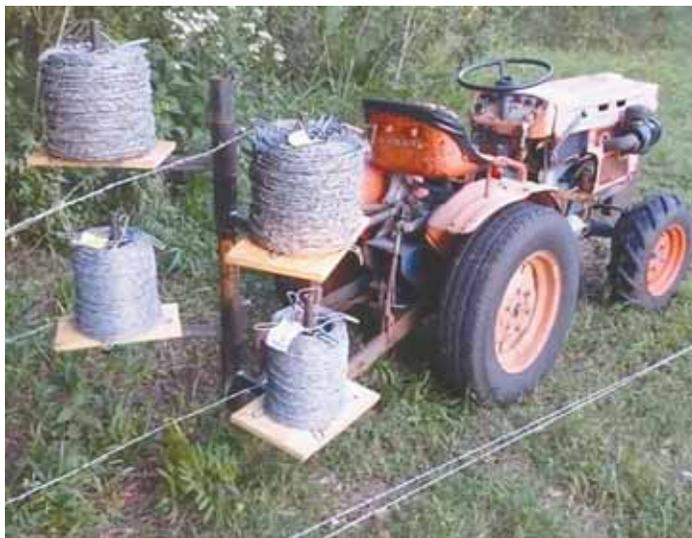
Short pieces of pipe, attached to small unrolling platforms, fit over main upright. Bass can unroll up to 6 wires at a time.
