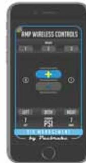
Smart phone app has 3 built-in memory presets to quickly adjust air spring pressure.
