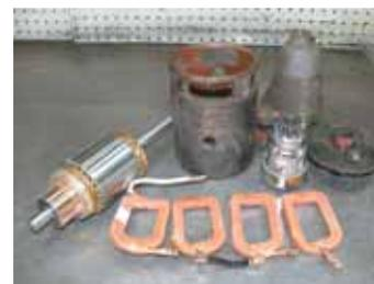
Photo shows Farmall M starter parts for conversion from 6 volts to 12 volts.
