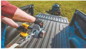
Using a cordless drill to power the Warn winch makes it truly portable.
