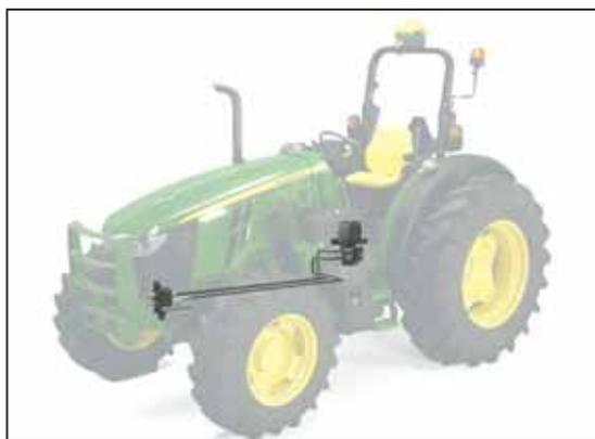
Deere says adding automated steering to your tractor, provided it has hydraulic steering, is easier and less expensive with its AutoTrac Controller 300.
