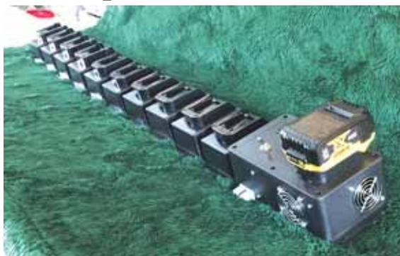
Multiple batteries can be recharged at one time with the aftermarket "Lion Charger" from Circuits Alive.
