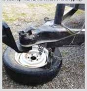
Steve Faber, Tiffin, Ohio: "I've found that I can easily break beads on tubeless tires using my trailer tongue jack. A short piece of bar stock placed along the edge of the rim makes it more effective."
