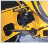
Marvin Martin, Elkton, Ky.: "On a Wrangler 4500 loader the hoses wanted to rub as they went through the frame at the articulation joint. I double wrapped the hoses with a piece of ratchet strap and secured them with zip ties temporarily. I then wrapped wire around the ratchet strap and tied it off, securing to the frame on one side. I used medium tension on the wires. I had to remove the front side access cover to reach the hoses."
