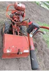
The coil on Podoll's rototiller was shot, but he got the machine going again by installing a 12-volt coil with bracket (below) and wiring it to a cordless tool battery strapped onto the handlebar.
