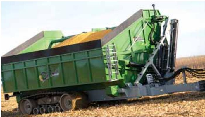
Brian Karg uses this 40-ton dump cart to haul sugar beets from his harvester to waiting trucks. It can empty its cargo in only about one minute.
