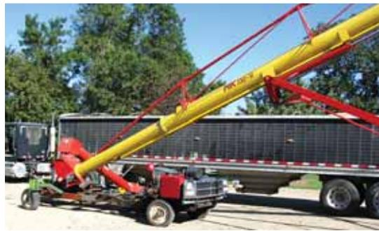
Ray Swenson built this self-propelled grain auger, equipped with a 91-ft. long swing-away auger, out of an old Dodge 4-WD pickup.
