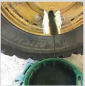
Loren Plett, Turpin, Okla.: "Ever try to drain a Honda engine with a pump mounted on it and not make a big oil spill? I used duct tape to make a channel for the oil to flow off to the side. Makes it easy to direct the oil where I want it to go and there's not much to clean up afterwards.
