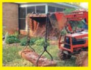
I beefed up the sides and top edge of my Kubota loader bucket with steel and then attached 3 hooks to the reinforced edge.
