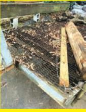
Another idea I had that works well is to use expanded metal on trailer decks. Gives good traction when loading a tractor and it helps firewood dry faster if I store it on there. Stringers underneath provide support. If I need a solid surface, I can put plywood over the metal. (John Rochester, Deerfield Beach, Fla.)
