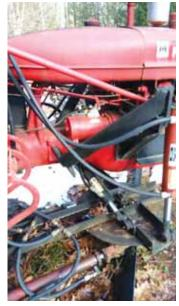
Cylinder between tractor frame and front crossbar controls blade movement.
