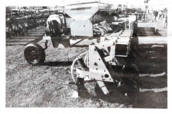
Drill attaches to the rear of cultivator with quick-tach levers, riding on a pair of caster wheels. Rig can be converted back quickly to straight cultivating.
