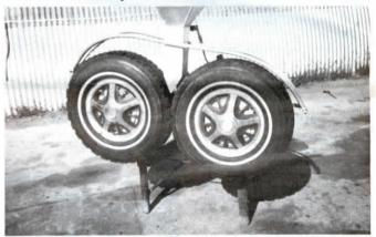
A pair of studded snow tires are used to flatten aluminum cans. Tires run up against each other, crushing cans down to about 1/4 in. thick.
