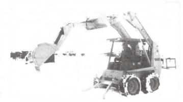
Backhoe snaps into quick-tach couplers on loader arms. Bucket is controlled by hydraulic cylinder powered by the skidsteer loader's auxilliary hydraulic system.
