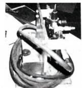
operate air tools at slower speeds so they won't wear out so fast, "We simply set the regulator at whatever pressure we want and lock it in place. The slower working speed also helps keep us from stripping sockets on our air impact wrenches."
