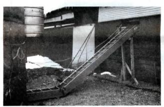
Haylage is dumped into the wooden elevator by a wagon on other side of silo and is mixed with corn silage delivered by silo unloader down a center discharge hole.
